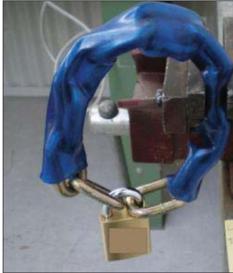
Figure 4: Padlock shackle vulnerability test setup
