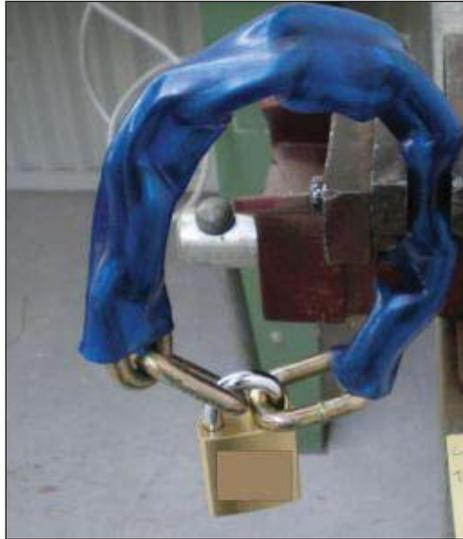
Figure 4: Padlock shackle vulnerability test setup
