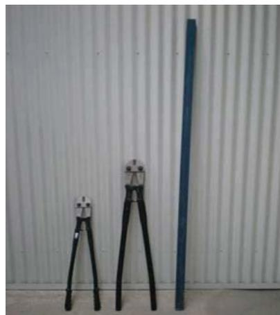
Figure 3. Vulnerability testing toolset, with 750mm bolt cutters on right.
