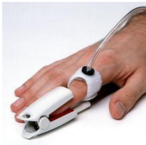
Fig. 2.5 – A pair of finger PPG sensors (Kirtley, 2002), wherein one is clipped to the top segment of the finger, and the other attached at the base of the finger. By measuring the transit time and the distance between the two points, PWV can be estimated.
