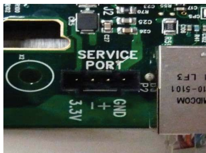
Figure 11. Service Port on a typical Air Handling Controller (AHC)
