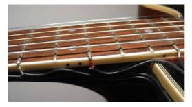
Figure 1. Cables soldered to the guitar frets
