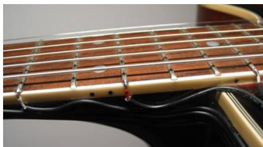
Figure 1. Cables soldered to the guitar frets
