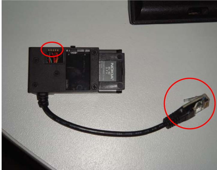
*Figure 7: Connectors on the UFS3 cable for Nokia 6600*
