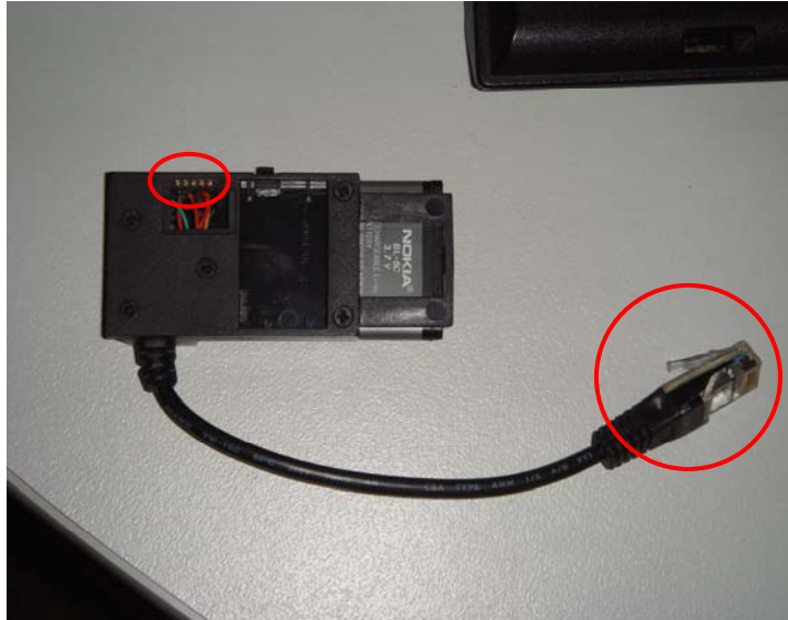
Figure 7: Connectors on the UFS3 cable for Nokia 6600
