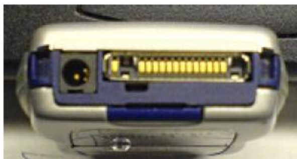
Figure 8: Nokia 3220 Fbus connections (Harrington 2007).
