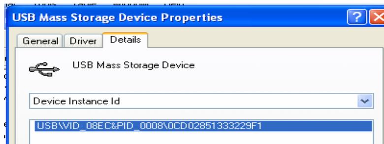
Figure 3. USB Device Instant ID as shown in device manager
