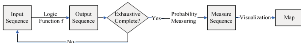
Figure 2: Flow Sheet of the Produce and Detect Mechanism of Time-Sequences
