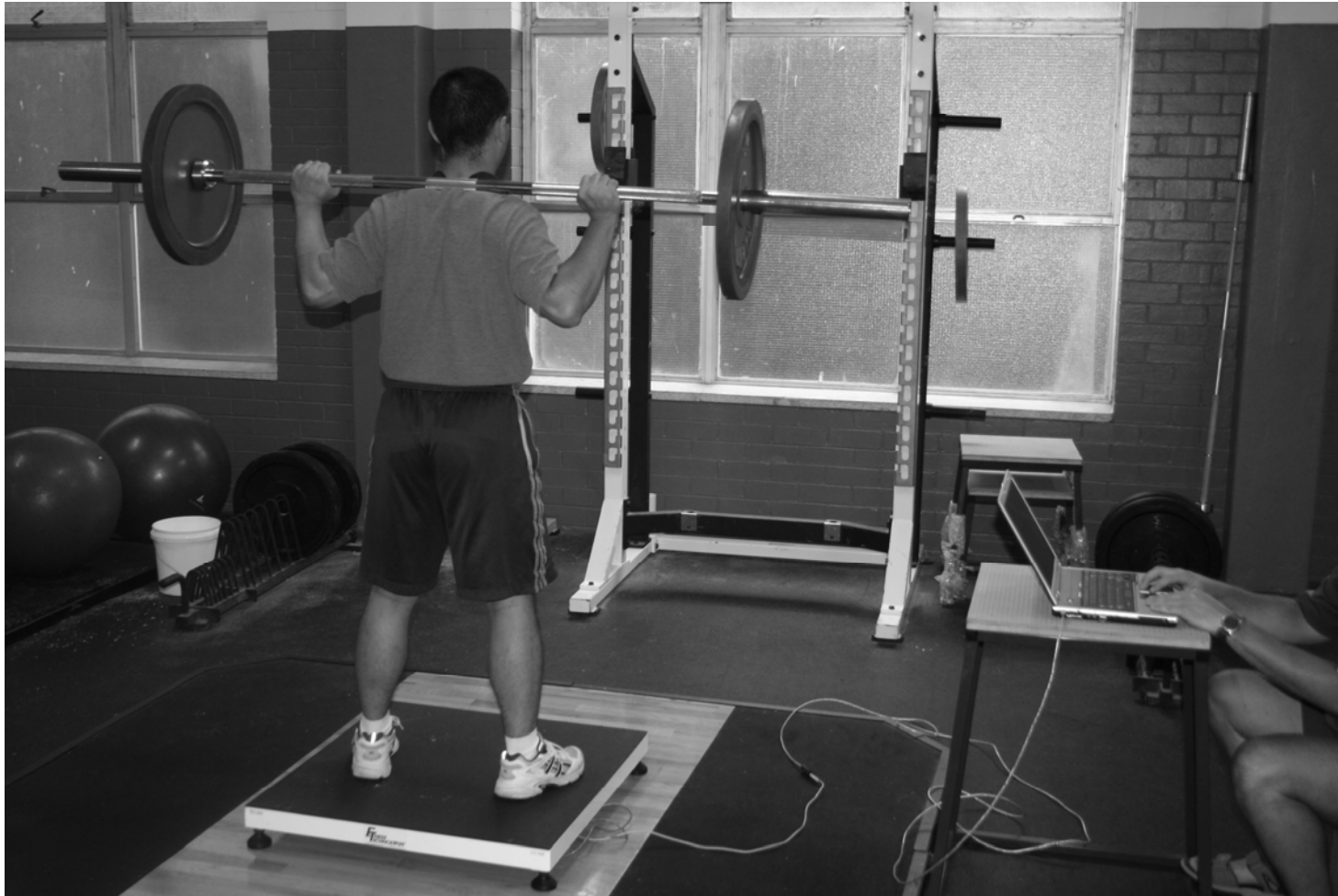
Figure 5.1 Experimental set up for weighted jump squat with measurement of ground reaction force.
