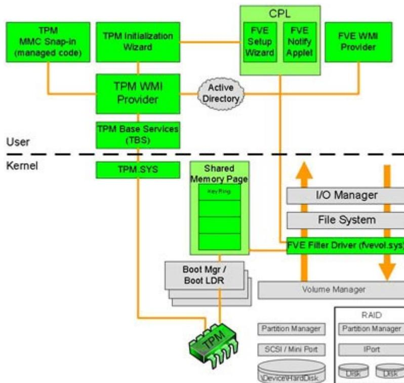
Figure 1: the overall BitLocker architecture (Microsoft 2006c)
