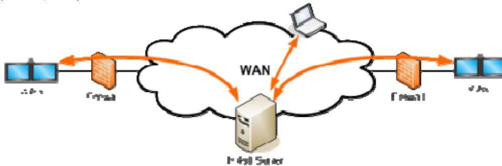
Figure 8. H.460 Server Used for Multimedia Tunnelling (Bartlett, 2008).
