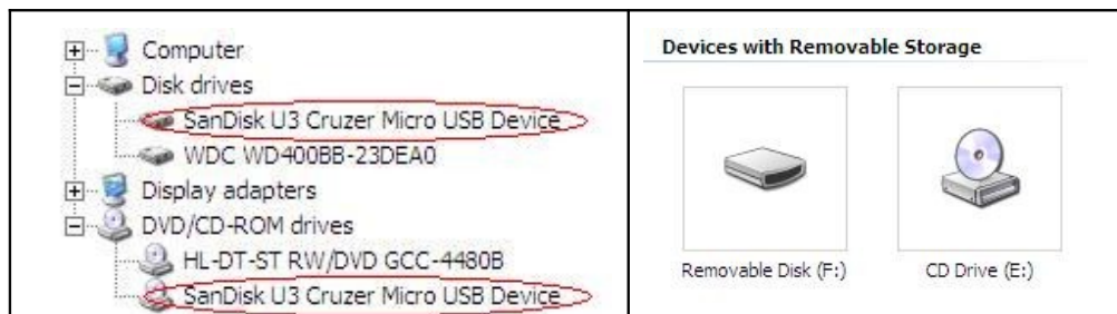
Figure 1: The two devices under device manager and as Removable Disk (F:) and CD Drive (E:)
