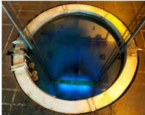
Figure 4.1 GATRI's cobalt-60 radioactive source [28].
