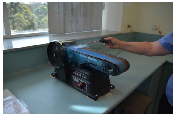
Figure 2: Effect of the Dust Extraction System for JBS Belt Sander and Buffer using Dräger Smoke Tube
