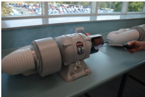
Figure 6: Effect of the Dust Extraction System for Redwing Sander/Grinders using Dräger Smoke Tube
