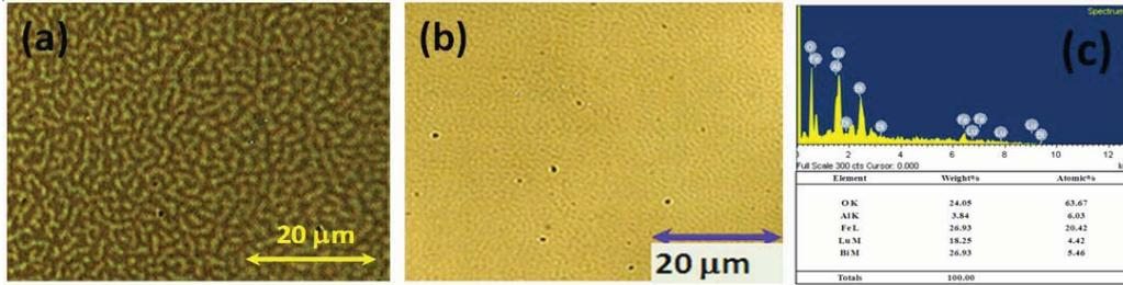
**Fig. 3:** Magnetic Domain Patterns Observed in Films Sputtered Onto GGG (111) at 250°C, Annealed for 1 h at 650°C (a); Deposited at 680°C and Annealed for 3 h at 630°C (b); and EDX Composition Measurement Data Obtained from Films Grown at 680°C Substrate Temperature
