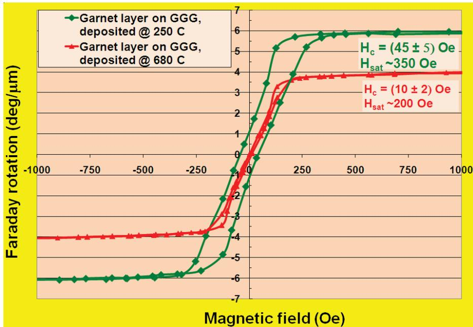
**Fig. 2:** Measured Hysteresis Loops of Specific Faraday Rotation at 532 nm in Sputtered  $\text{Bi}_{1.8}\text{Lu}_{1.2}\text{Fe}_{3.6}\text{Al}_{1.4}\text{O}_{12}$  Garnet Films on GGG Substrates Deposited at (a) 250°C and Annealed for 1 h at 650°C, and (b) 680°C Substrate and Annealed for 3 h at 630°C.
