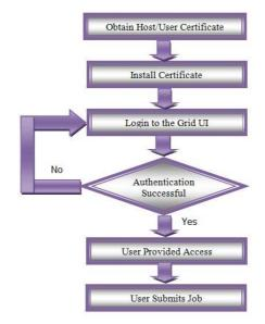
Figure 2: Process of Accessing Grid System
