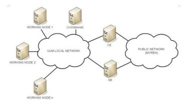
Figure 1: Architecture of the Sintok-Grid
