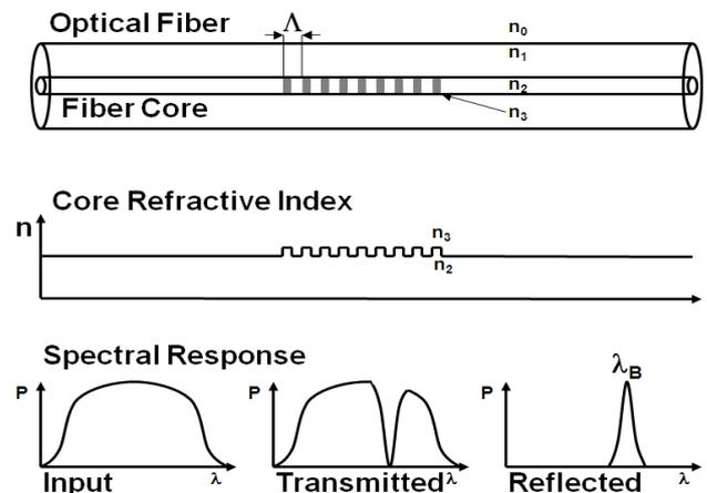
Figure 1. FBG fundamental principle of operation [3].
