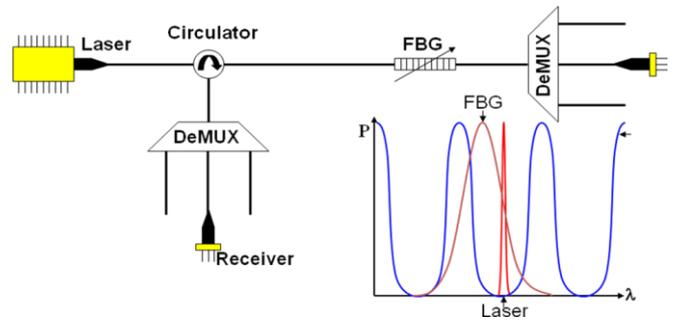
Figure 3. Optical circuit with principle of operation.
