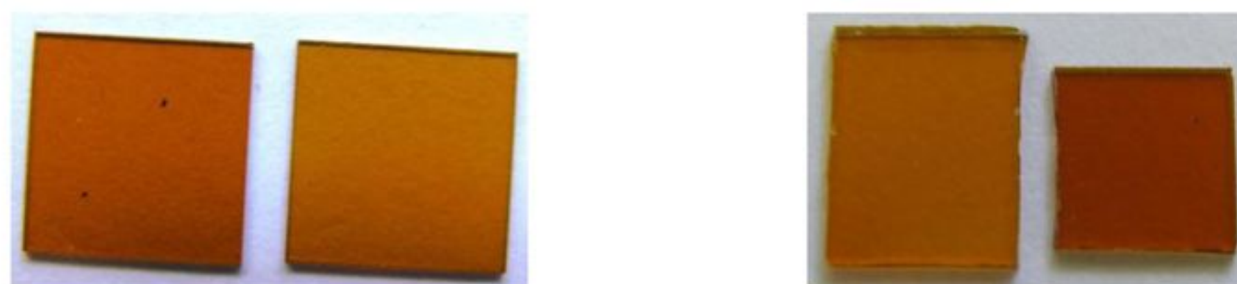
Fig. 1 (a) Left: 650-nm-thick film of \text{Bi}_{1.8}\text{Lu}_{1.2}\text{Fe}_{3.6}\text{Al}_{1.4}\text{O}_{12} on a \text{Gd}_3\text{Ga}_5\text{O}_{12} (GGG) substrate; Right: 1150-nm-thick film of (\text{Bi}_{1.8}\text{Lu}_{1.2}\text{Fe}_{3.6}\text{Al}_{1.4}\text{O}_{12} + 20 \text{ vol } \% \text{ co-sputtered } \text{Bi}_2\text{O}_3) on a GGG substrate (both films are as-deposited); (b) Left: 1030 nm (\text{Bi}_2\text{Dy}_1\text{Fe}_4\text{Ga}_1\text{O}_{12}:\text{Bi}_2\text{O}_3 \text{ 24 vol } \%) on glass, after 2 h @ 580 °C, Right: 1080 nm \text{Bi}_2\text{Dy}_1\text{Fe}_{4.3}\text{Ga}_{0.7}\text{O}_{12} on GGG, after 1 h @ 700 °C.
