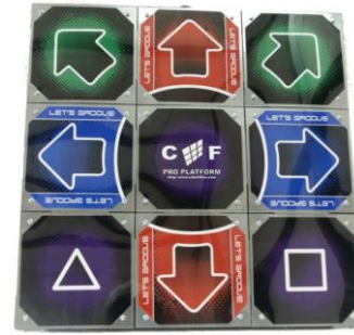
Figure 1: A dance pad produced by Cobalt Flux. The pad rests on the floor and is divided into a number of areas (9 in the shown pad), each area acting as a switch.
