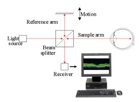
Fig. 1 Operating principle of a Michelson interferometer type OCT system.
