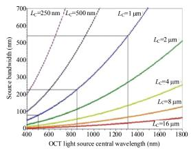
Fig. 2 Free space OCT iso-resolution lines (iso-LC lines); bandwidths for typical OCT sources (generation based on Fig. 8.2 of [2]).
