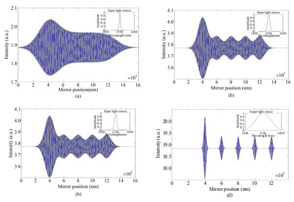
Fig. 3 OCT interferogram A-scan of a five-layer virtual sample (each layer is 100 µm thick) with the associated source spectrum insert: source bandwidths are (a) 10 nm, (b) 20 nm, (c) 50 nm, and (d) 100 nm, with the central source wavelength of 1550 nm.
