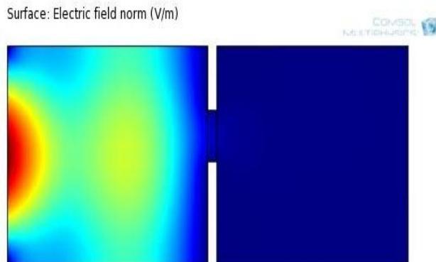
**Fig. 4. Electric field density for PANi shielding device**
