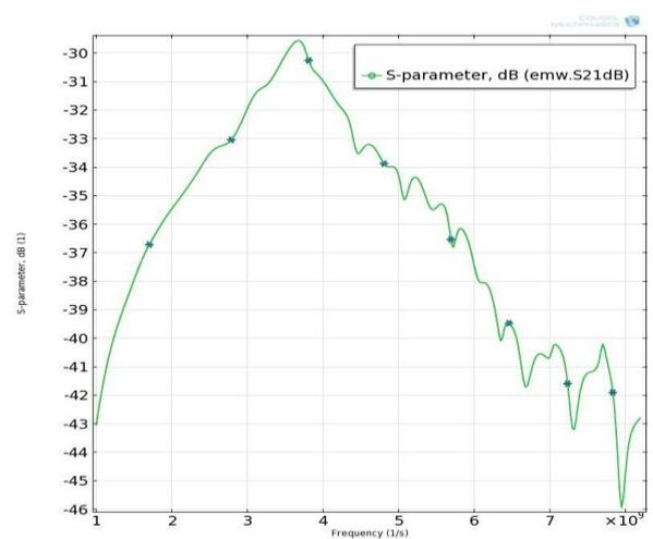
**Fig. 5. Transmission loss S21 for PANi shielding device**
