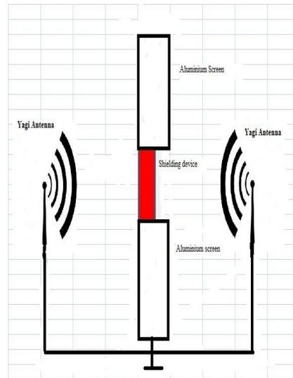
**Fig. 2. Experimental set up**
