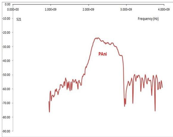
**Fig. 3. PANi Transmission losses**
