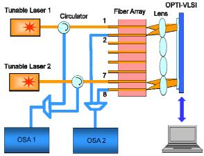
Fig. 7. Experimental setup to demonstrate the concept of the photonic RF signal processor.
