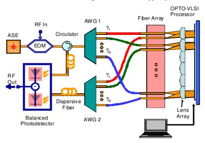
Fig. 3. Proposed reconfigurable photonic RF filter based on an Opto-VLSI processor and a 4f imaging system.
