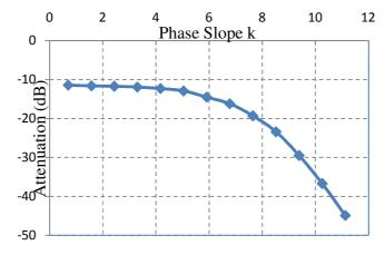
Fig. 10. Attenuation versus phase slope of holograms uploaded onto the Opto-VLSI processor
