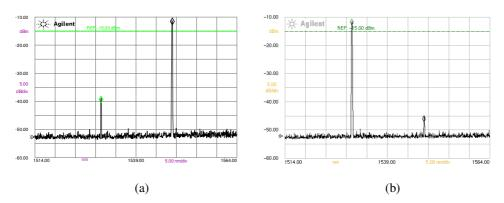
Fig.9. Experimental results showing the incident signals can be controlled for positive and negative weights. (a) The signal with wavelength  $\lambda_1$  was steered for positive detection; (b) the signal with wavelength  $\lambda_2$  was steered for negative detection.
