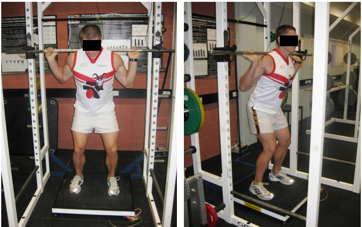
Figure 1. Frontal and side view of set-up and operation for the fixated isometric apparatus.
