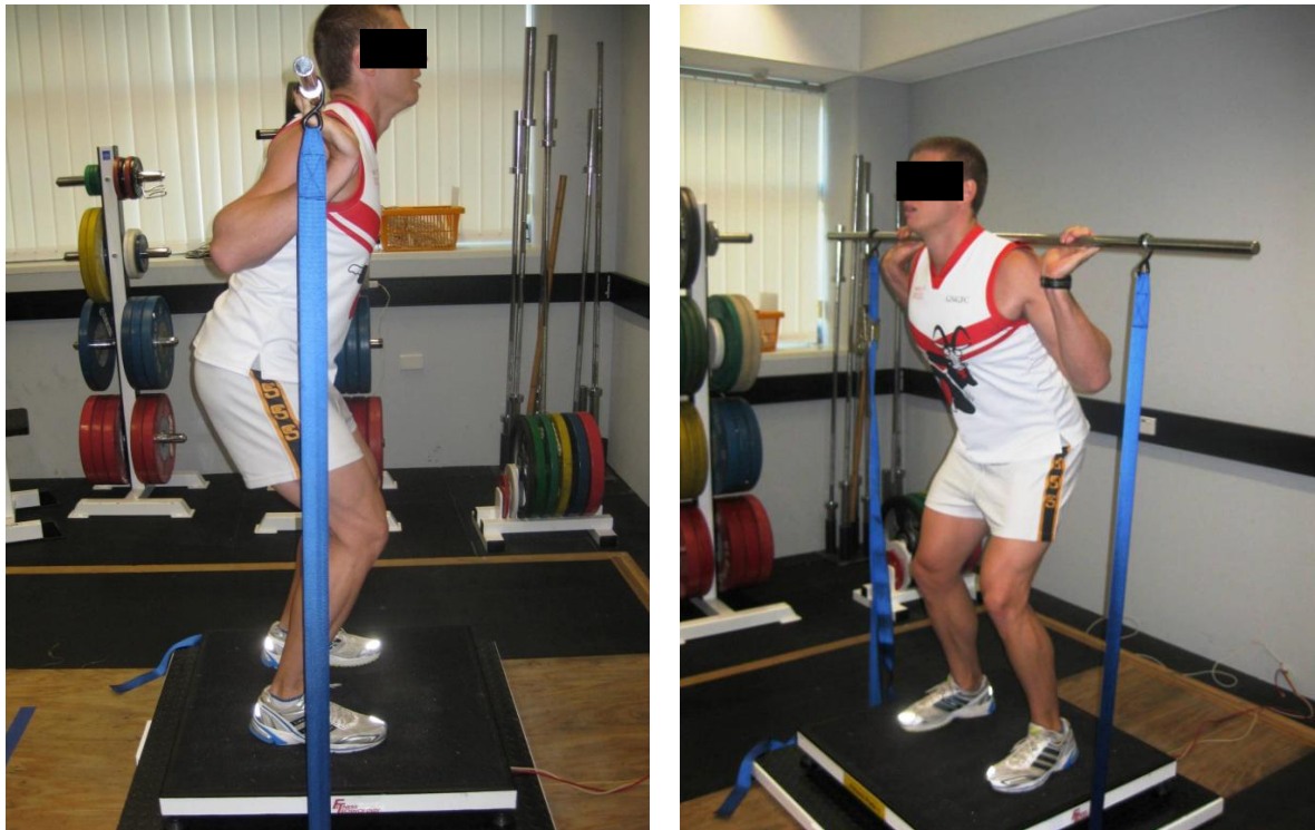
Figure 2. Frontal and side view of set-up and operation for the portable isometric apparatus.
