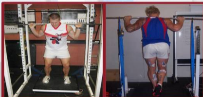
Figure 1. Fixated (left) and portable (right) isometric strength assessment devices comparing bilateral and unilateral squat positions.
