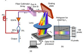
Fig. 1. Opto-VLSI-based tunable fiber laser structure. PC: polarization controller.
