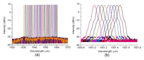
Fig. 3. Measured outputs of the Opto-VLSI-based fiber laser. (a) Coarse wavelength tuning over C-band, and (b) fine wavelength tuning.
