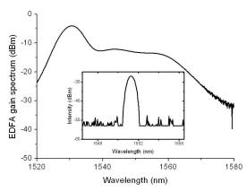
Fig. 2. Amplified spontaneous emission (ASE) noise from the EDFA. The inset is an example of a waveband selected by the Opto-VLSI processor.
