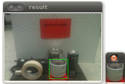
Figure 7. Object detection by template matching technique: original image is on the left and template image is on the right.
