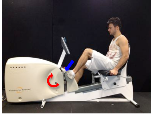
Figure 1.1: Eccentric cycling ergometer (Eccentric trainer, Metitur, Finland). The red-circled arrow represents the backward rotational movement of the cranks, and the blue-straight arrow represents the force applied by the subject to resist the crank movement.
