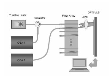
Fig. 3. Experimental setup for demonstrating the concept of the ROAD structure shown in Fig. 2.
