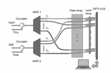
Fig. 2. Novel ROADM structure employing AWGs, a custom-made fiber array, and an Opto-VLSI processor for optical beam steering.
