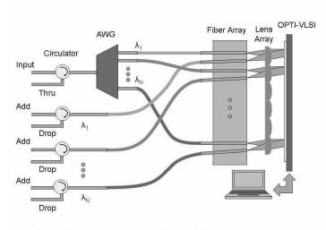
Fig. 5. A ROADM structure with multiple add/drop ports.
