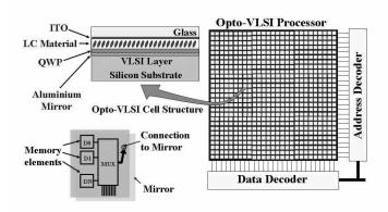
Fig. 1. Opto-VLSI processor structure
