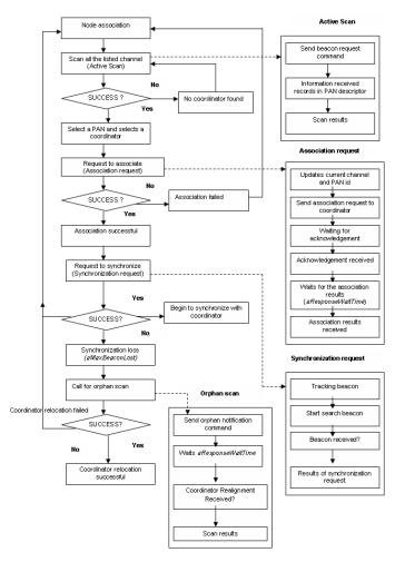
Fig. 3. Flow of node association and synchronization
