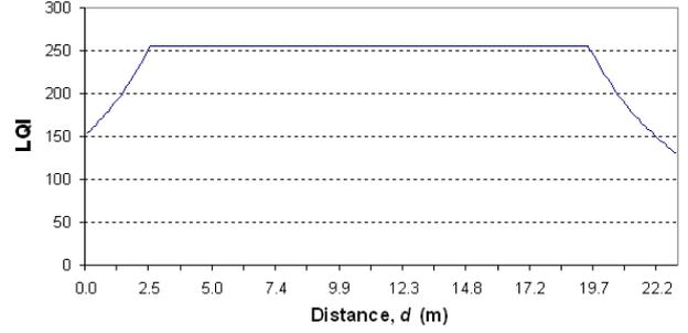
Fig. 2. LQI for a node moving across the center of the coverage area
