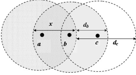
Fig. 4. Three coordinators with overlapping radio coverages
