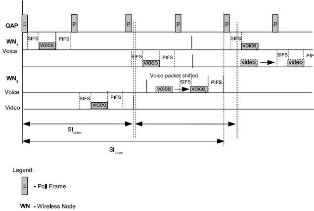
Fig. 6. Frame Exchange of Voice and Video Packets
