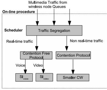
Fig. 5. Main optimizing architectures implemented in QAP
