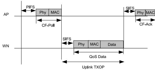
Fig. 3. Basic Frame Exchange in CFP
