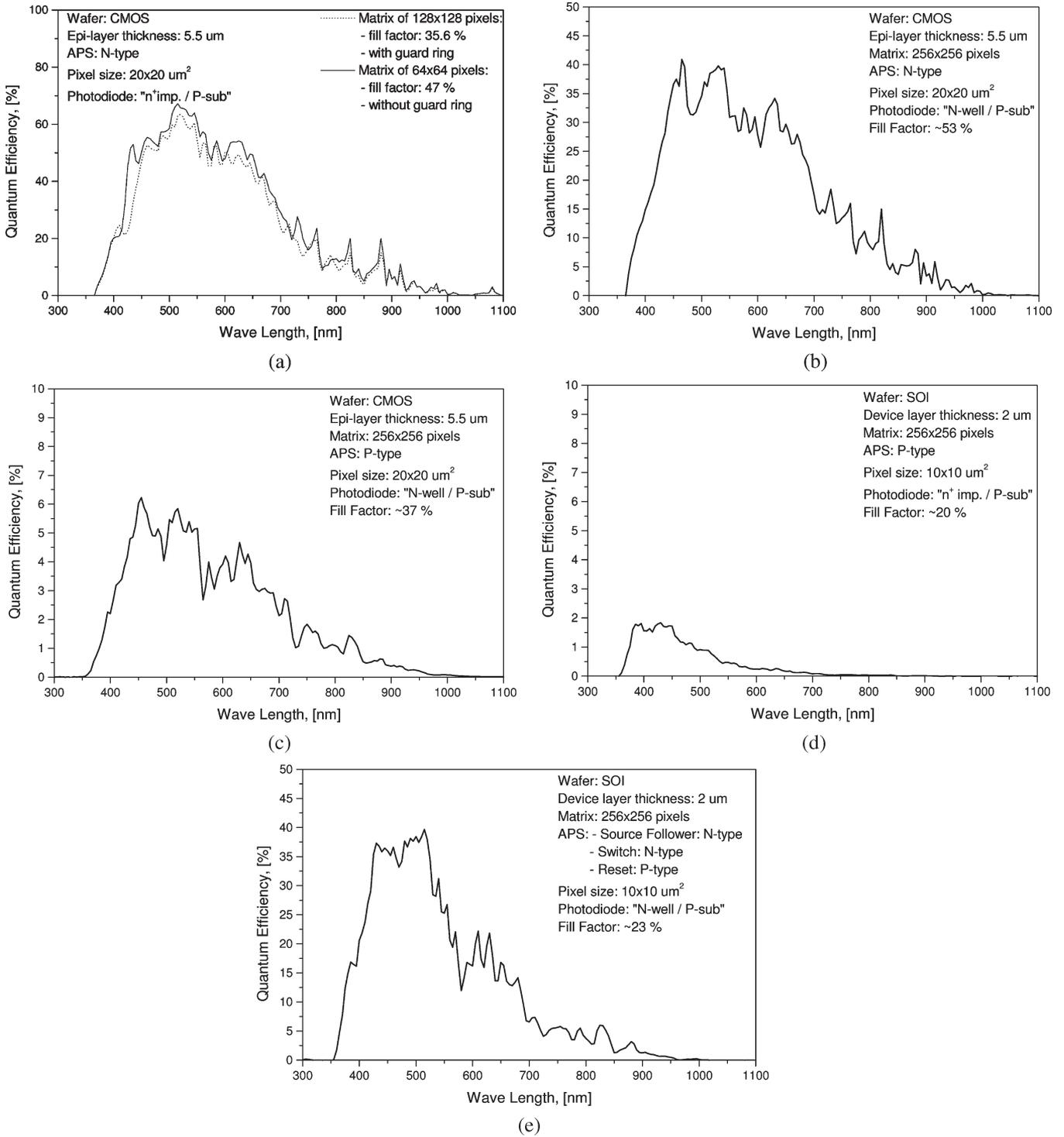
Fig. 3. Measured quantum efficiency for (a) “Imager-1” and “Imager-2,” corresponding to Fig. 2(a) and (b); (b–c) “Imager-3” and “Imager-4,” corresponding to Fig. 2(c) and (d); and (d–e) “Imager-5” and “Imager-6,” corresponding to Fig. 2(e) and (f).
