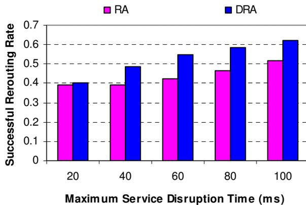
Fig. 7: Successful rerouting rate for various time limits.
