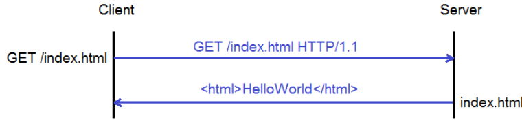
Figure 2-4: An end-to-end HTTP communication
