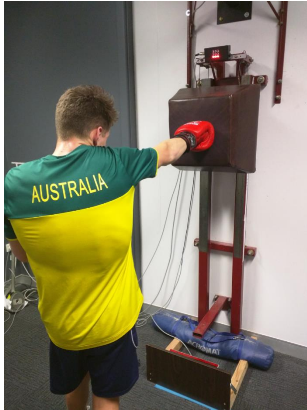
Figure 8.1 The punching integrator device collects peak impact punching forces and velocity prior to impact.
