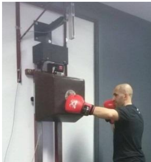
Figure 5.1 Image of a participant punching the punching integrator device. The punching integrator device collects peak impact punching forces and velocity prior to impact.
