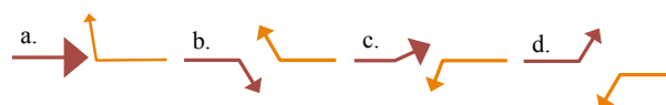
Figure 4. Collision avoidant using force evaluation: a. strong(L)/weak(R) interaction, b. weak(L)/weak(R) interaction, c. medium(L)/weak(L) interaction, and d. spatially higher stream deflects lower stream downwards.
