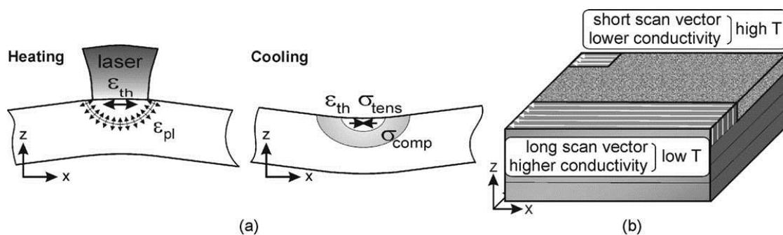
Fig. 2.23 The thermal deformation mechanism during the melting process [15]
