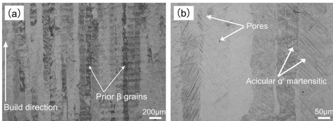
Fig. 2.26 SLM optical image of Ti-6Al-4V at the vertical direction[106]
