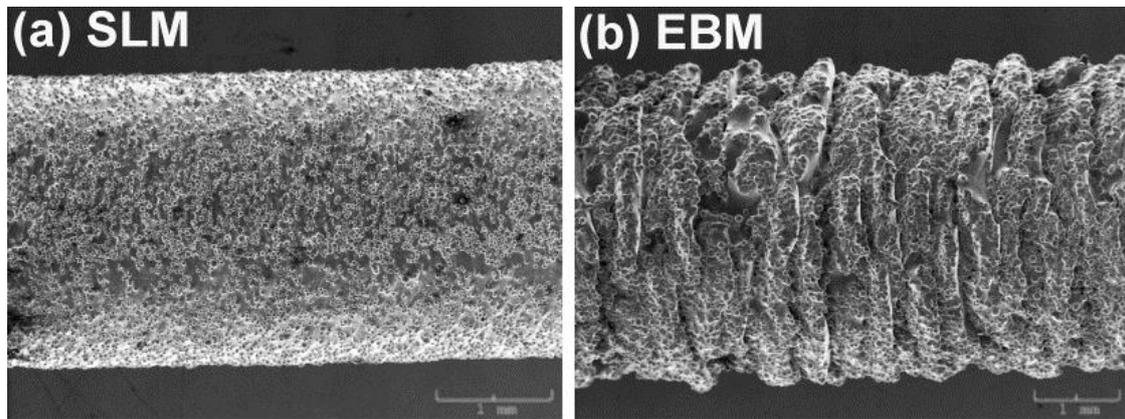
Fig. 2.20 The surface view of the SLM- and EBM-produced Ti-6Al-4V samples [80]
