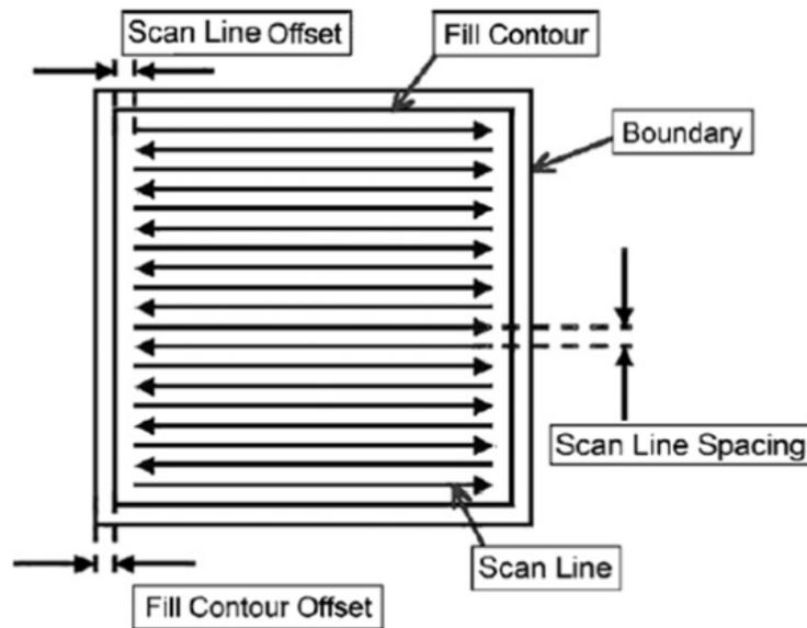
Fig. 2.17 Definition of Scan Spacing[68].
