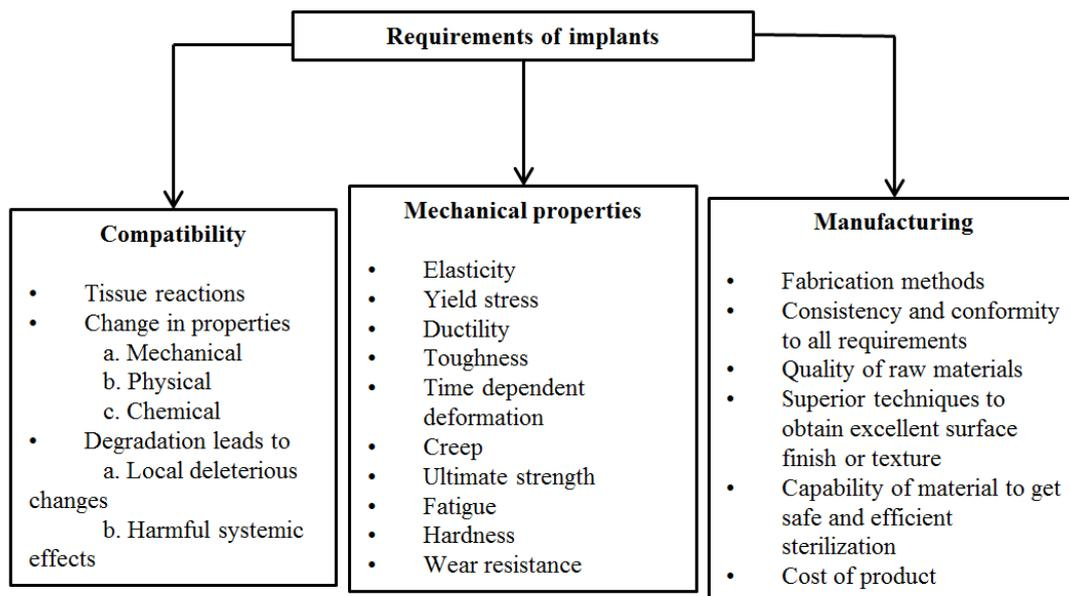
Fig. 2.1 Implant requirements in orthopaedic applications.
