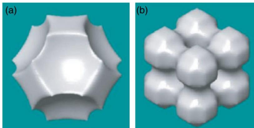
Fig. 2.10 Architectural design of scaffold unit based on geometric equations[49].
