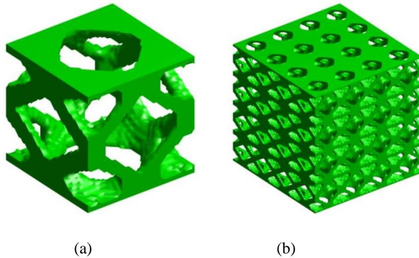
Fig. 2.12 Scaffold unit and structure by using solid freeform fabrication (SFF) for researching the relationship between the stiffness and remodelling in (a) the unit of scaffolds and (b) a scaffold base cell in a  $4 \times 4 \times 4$  structure [51].
