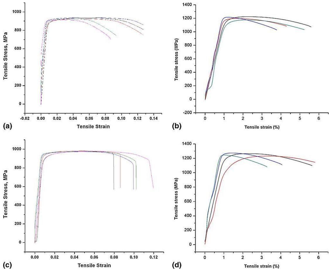
Fig. 2.30 Stress-Strain plots of Ti-6Al-4V specimens, (a) EBM specimen built in building direction, (b) SLM specimen built in building direction, (c) EBM specimen at x-y cross section and (d) SLM specimen built at x-y cross section[109].
