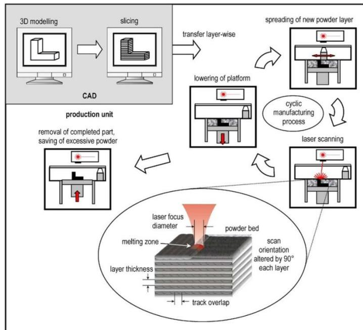
Fig. 2.14 Schematic illustrating the additive manufacturing process [54]
