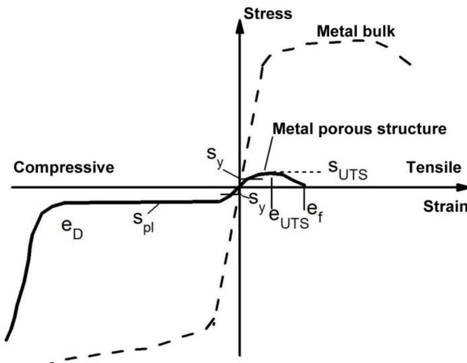
Fig. 2.7 A comparison of the stress-strain curves between the metal solids and the porous structure [30].
