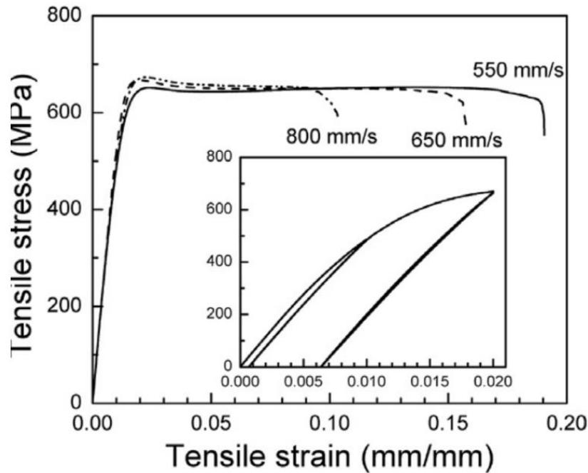
Fig. 2.6 Typical stress–strain curves of parts processed at laser scan speeds of 550, 650 and 800 mm/s [7].
