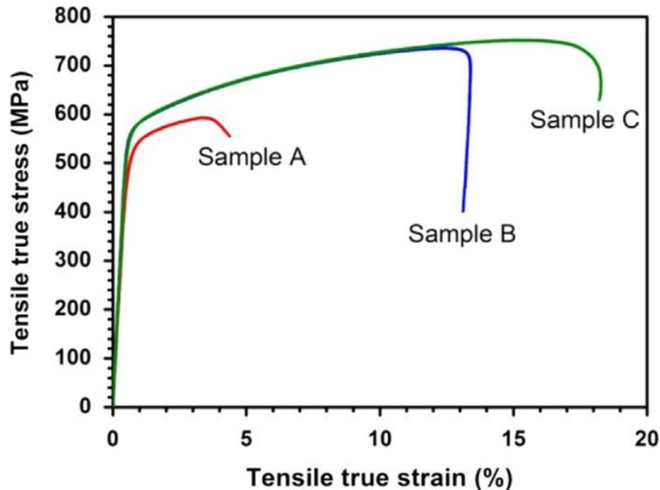
Fig. 2.29 The tensile stress-strain curves of the CP-titanium samples for SLM-produced (Sample A:  $P=85\text{W}$ ,  $v=71\text{mm/s}$ , and relative density= $96.4\%$ ; sample B:  $P=135\text{W}$ ,  $v=112\text{mm/s}$ , and relative density= $98.7\%$ ; and sample C:  $P=165\text{W}$ ,  $V=138\text{mm/s}$ , and relative density= $99.5\%$ ) [108].
