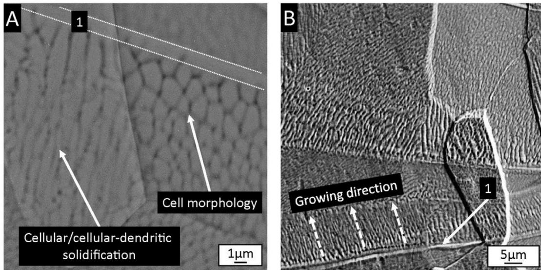
Fig. 2.25 The morphology of cellular/cellular-dendritic in the near- $\beta$  titanium alloy Ti-5553[105].
