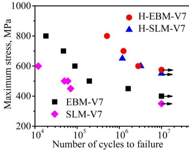
Fig. 2.31 S-N curves of AM-produced samples and HIP Ti-6Al-4V samples
