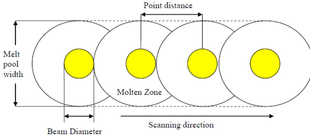
Fig. 2.16 Illustration of Point Distance Beam Diameter and Melt Pool Width.
