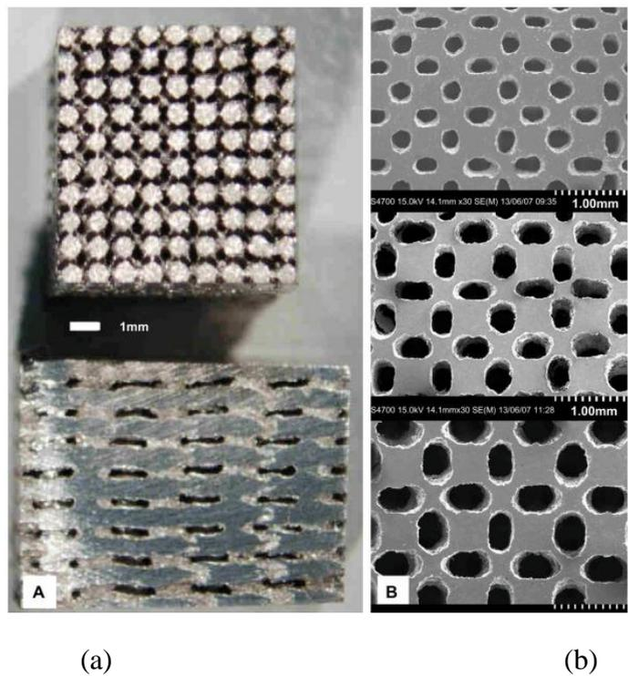
Fig. 2.13. 60% porosity scaffold template model and titanium scaffolds with 200µm to 400µm pore size [52].
