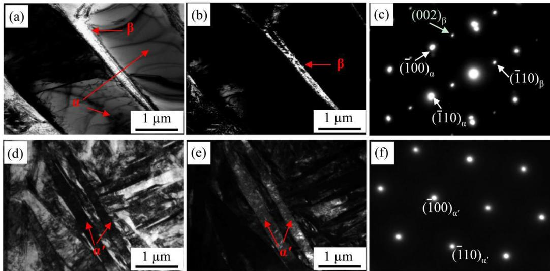
Fig. 2.27 The TEM image of the SLM and EBM for Ti-6Al4-V alloy [107]
