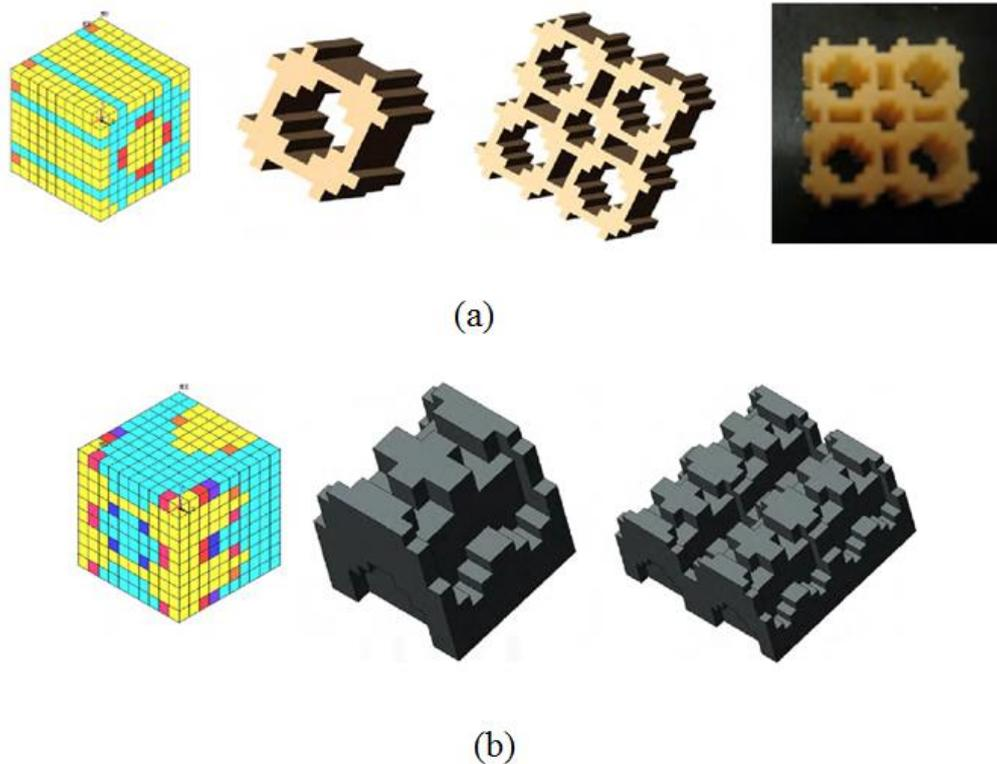
Fig. 2.11 Picture of 50% porosity scaffold structure using additive technologies [50].
