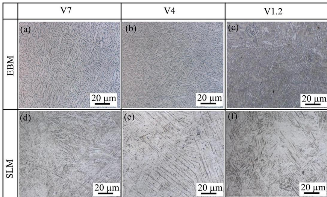
Fig. 2.28 The optical image of the SLM and EBM for Ti-6Al-4V [107]
