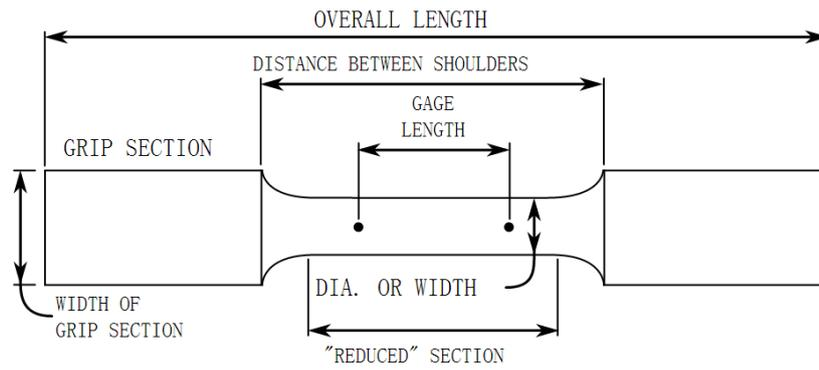
Fig. 2.5. The tensile specimen structure.
