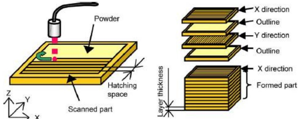
Fig. 2.18. Illustrating Layer Thickness [69].
