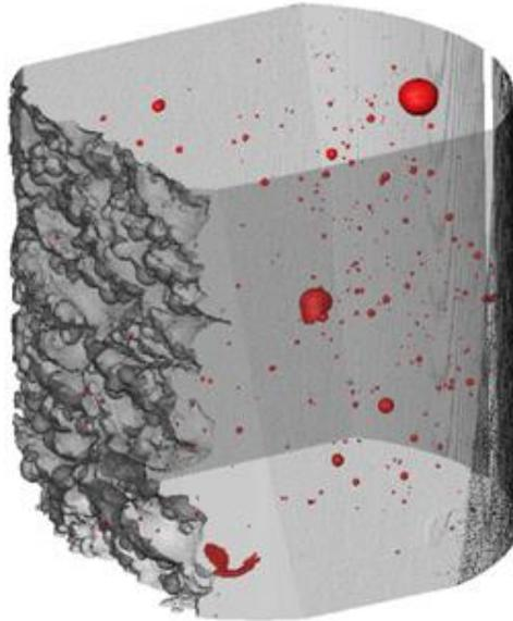
Fig. 2.22 Micro-CT image of the size and distribution of the defect pores [94].
