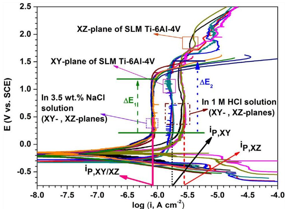
Fig. 2.33 The potentiodynamic curves for the x-y and x-z cross section plane of AM-produced specimens
