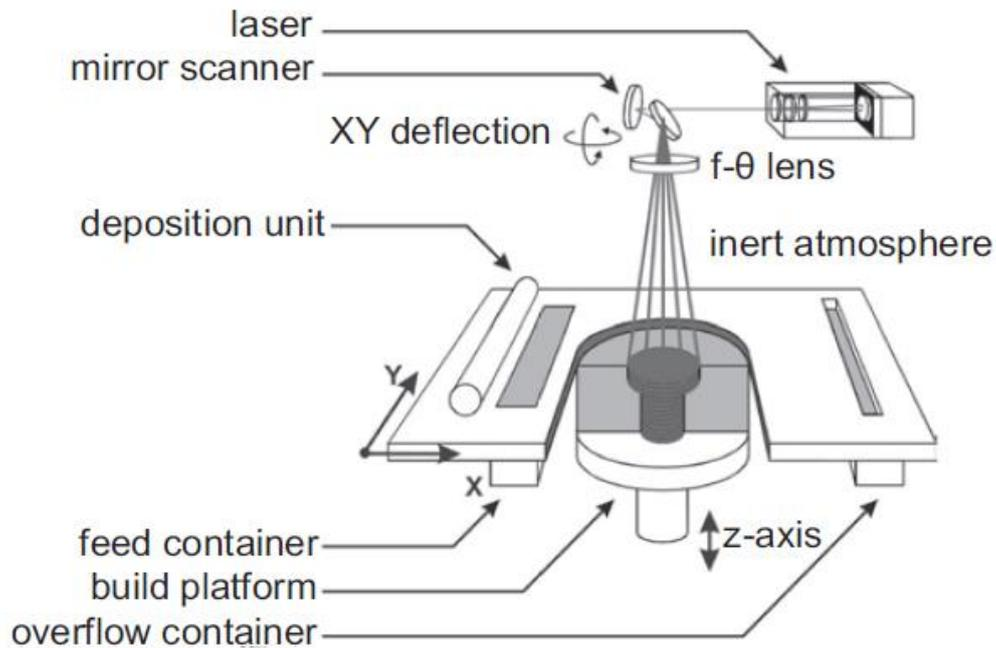
Fig. 2.15 The schematic of the SLM building process[65].
