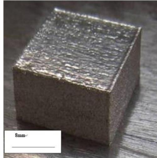
(b) the SLM fabricated entity
