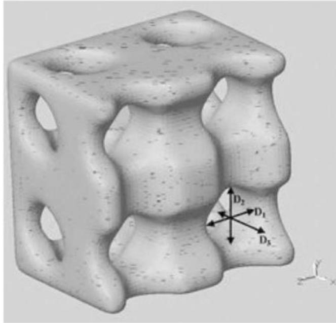
Fig. 2.9 The image of a scaffold unit with pores designed by a computer and in-grown bone cells [48].
