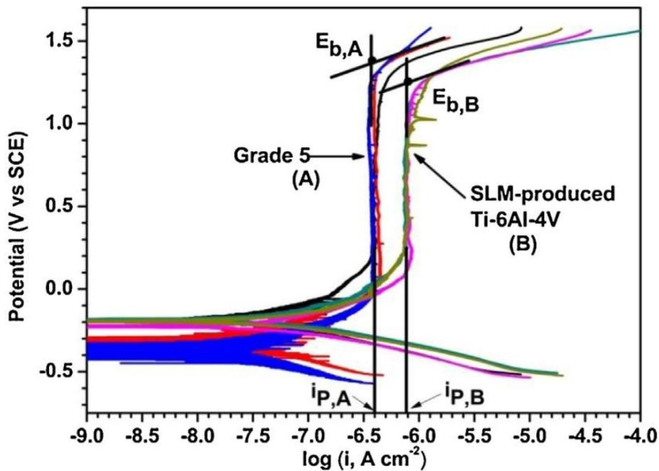
Fig. 2.32 The Potentiodynamic curves for the SLM-produced Ti-6Al-4 V alloy and commercial Grade 5 alloy in 3.5 wt.% NaCl solution [106].
