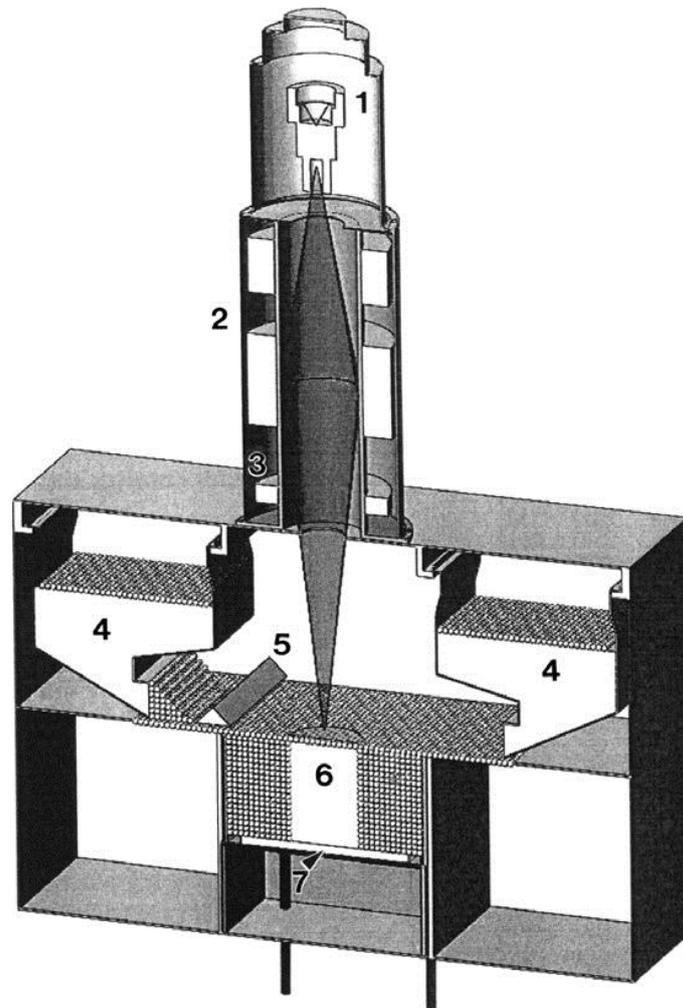
Fig. 2.19 The schematic rendering of EBM system [79].
