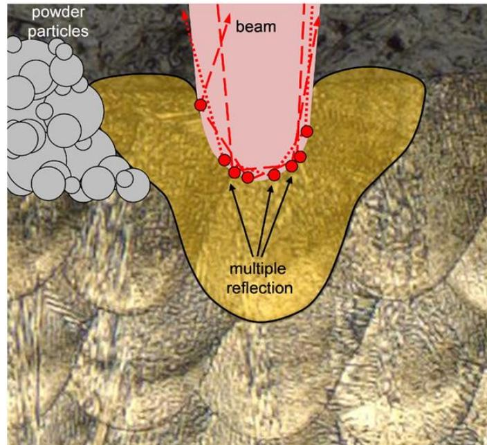
Fig. 2.24 The process of the SLM melting, within these keyholes, multiple reflections, absorption at the keyhole walls occur[104].
