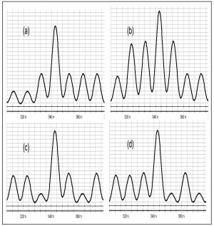
**Figure 3.** Parametric faults of the variable gain amplifier, (a) The first Amplifier output voltage < 1.2mV; fault detected. (b) The second Amplifier output voltage equal 2mV, fault detected. (c) The third Amplifier output voltage < 1.2mV; fault detected. (d) The fourth Amplifier output voltage < 1.2mV; fault detected.
