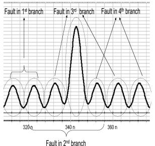
Figure 4. Optical correlator output signature
