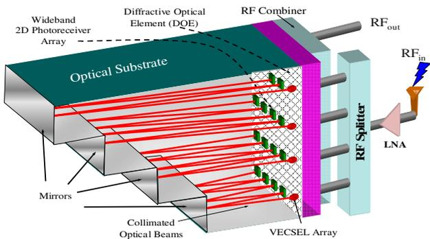
Figure 3. Architecture of the MicroPhotonic RF filter
