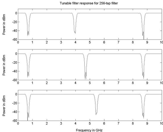
Figure 6. Three-band MicroPhotonic filter responses. Tuning around 4.75 GHz.
