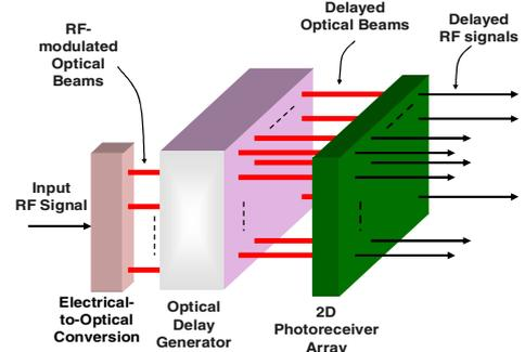
Figure 2. Principle of MicroPhotonic RF signal processing
