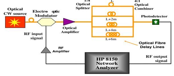
Figure 1. The configuration of conventional photonic RF filter
