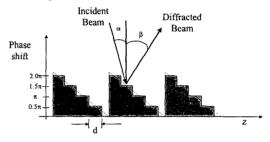
Figure 2. 4-phase stepped blazed grating structure.
