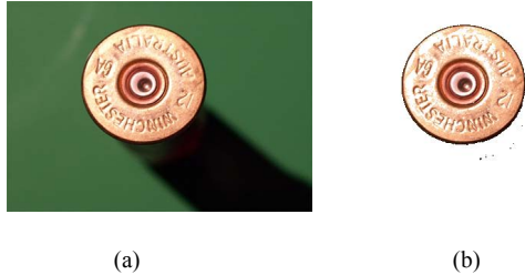
Fig. 7 Remove the background and shadows. (a) Input image, (b) Result removed background and shadows
