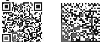
Figure 1. An example of QR Code (left) and Data Matrix (right) symbologies.
