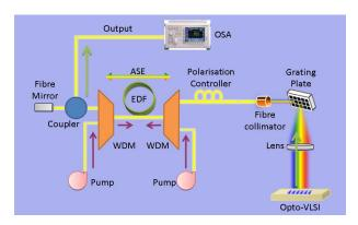
Figure 3. Architecture of the fibre laser employing an Opto-VLSI processor.
