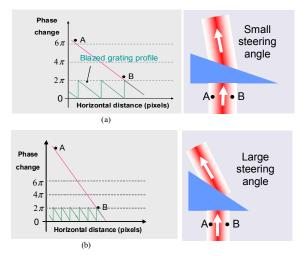
Figure 2 (a) and (b). Comparison of different blaze grating profiles versus the corresponding phase change.
