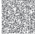
Fig. 6. An example of the monochrome QR Code compressed using the baseline JPEG scheme in our experiment.
