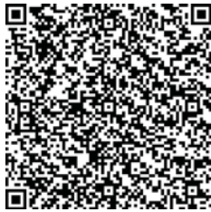
Fig. 17. QR code with message size of 240 bytes and 27% error correction ability
