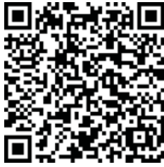
Fig. 15. QR code with message size of 70 bytes and 27% error correction ability
