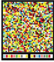
Fig. 13. Physical size of the MMCC code used in this paper, 30 mm by 33.75 mm
