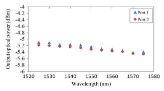
Fig. 8. Measured output power at ports 1 and 2 versus wavelength for a splitting ratio = 1.0.
