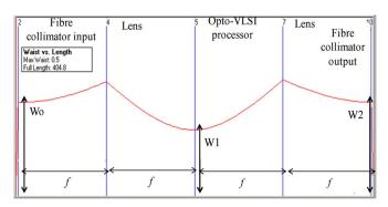
Fig. 4. Simulation results showing the optical beam waist along the 4-f imaging system. W0 is the input beam waist at the input fiber collimator, W1 is the beam waist at the Opto-VLSI processor, and W2 is the waist of the reflected beam as it reaches the output fiber collimator.
