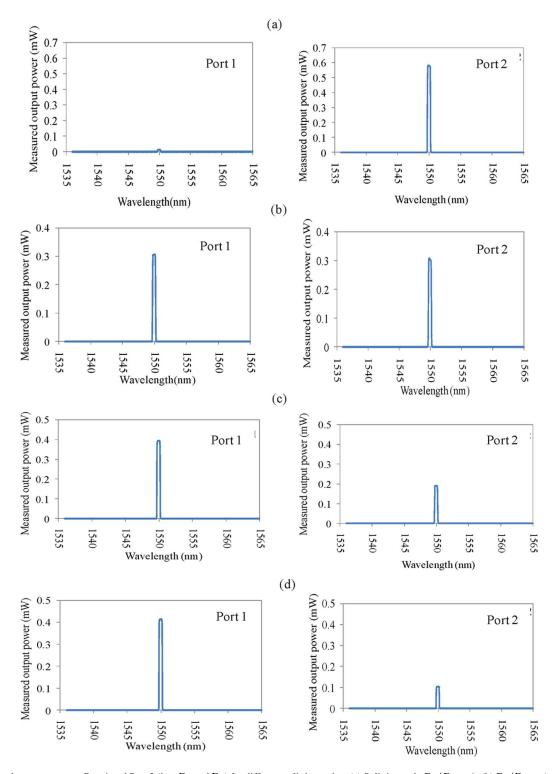
Fig. 5. Measured output power at Port 1 and Port 2 (i.e.,  $P_1$  and  $P_2$ ) for different splitting ratios. (a) Splitting ratio  $P_1/P_2=0$ , (b)  $P_1/P_2=1$ , (c)  $P_1/P_2=2$ , and (d)  $P_1/P_2=4$ .
