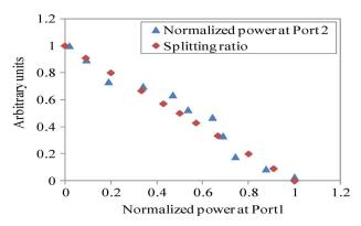
Fig. 7. Normalized output power at Port 2 ( $\blacktriangle$ ) and the corresponding splitting ratio (arbitrary units) ( $\spadesuit$ ) versus the normalized power at Port 1.
