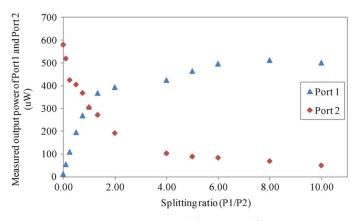
Fig. 6. Measured output powers at Port1 ( $\blacktriangle$ ) and Port 2 ( $\spadesuit$ ) versus the splitting ratio  $(P_1/P_2)$ .
