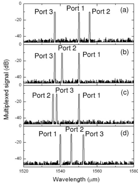
Fig. 2. Multiplexing operation of the proposed adaptive multi/demultiplexer
