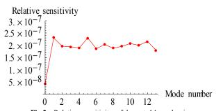
**Fig.2** Relative sensitivity of lowest 14 modes in PCF. Mode number 0 is the fundamental core mode.
