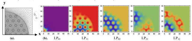
Fig. 1 (a). Meshed PCF geometry, due to the symmetry nature of PCF, the quarter cross-section is divided into a patchwork of triangular elements. Silica index =1.45, Pitch  $\Lambda = 9.7 \mu m$ , air-hole diameter d = 0.42  $\Lambda$ , Outer PCF diameter =83 $\mu$ m (b).  $E_x$  is the field distribution obtained for the fundamental core mode and the first four cladding modes in PCF by SFEM at  $\lambda$ =1560 nm.
