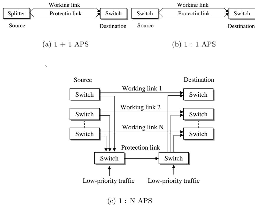
Figure 2.4: Automatic protection switching
