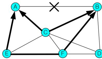
(c) Failure of Straddling link
