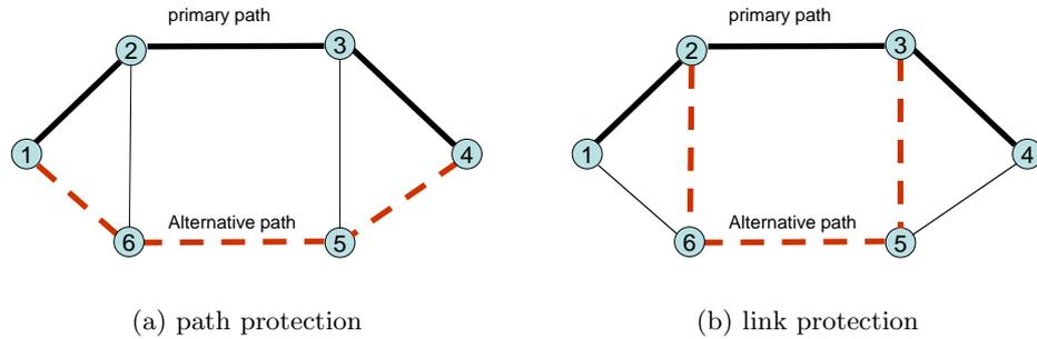
Figure 2.6: Two basic survivability mechanisms in mesh networks
