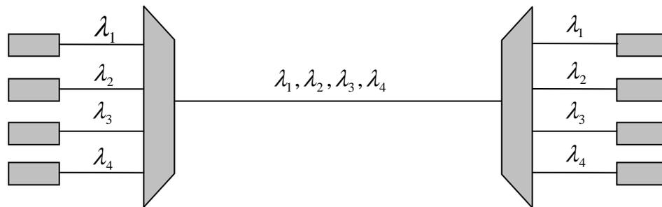
Figure 2.1: *Configuration of a basic WDM transmission system*
