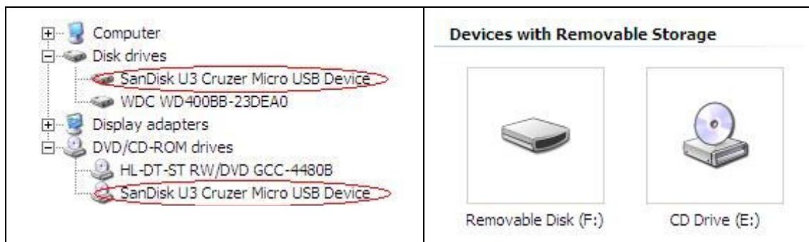
Figure 1: The two devices under device manager and as Removable Disk (F:) and CD Drive (E:)
