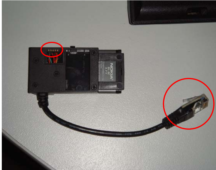
Figure 7: Connectors on the UFS3 cable for Nokia 6600
