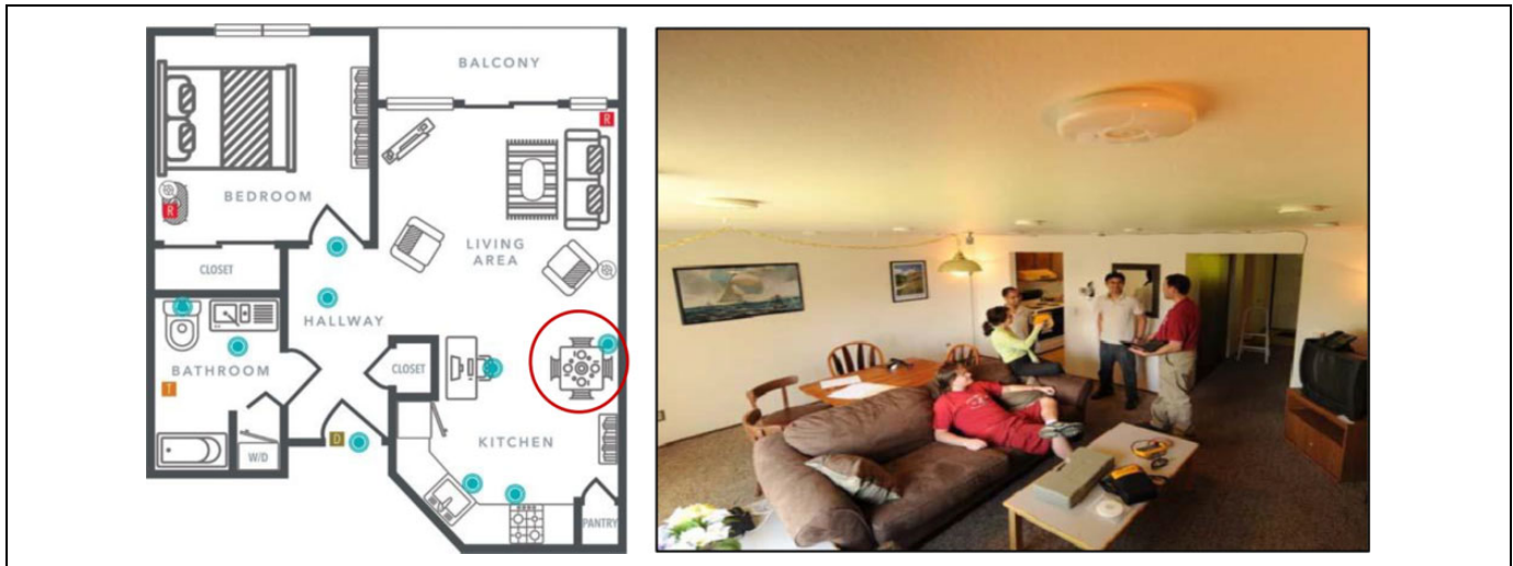
Figure 1. Floor plan with sensor locations identified in blue, red, and green (Left). Sensors installed in a residence; the Center for Advanced Studies in Adaptive Systems (CASAS) smart home testbed; Washington State University campus, Pullman, WA, USA (Right).
